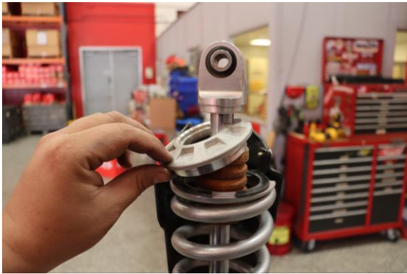
Step 21. Install the OE lower spring perch.
