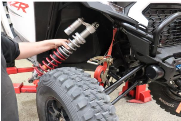
Step 17. Install shock assembly in the vehicle.
