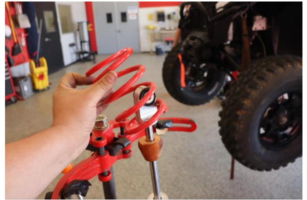
Step 10. Remove the OE tender spring.
