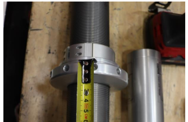
Step 12. Install Eibach crossover ring and adjust until it contacts the upper spring perch. The crossover ring is inactive in this install.
