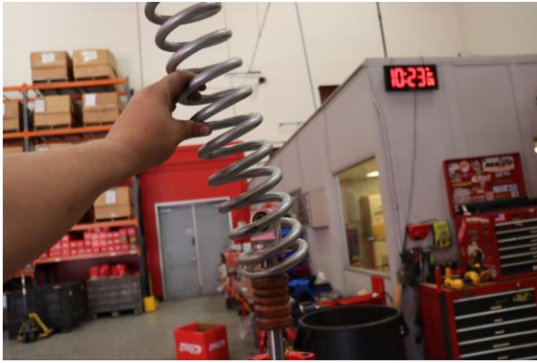
Step 19. Install Eibach main spring.
