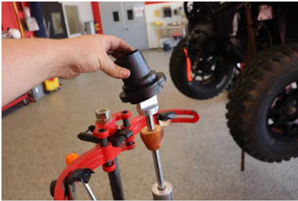
Step 9. Remove the OE spring slider.
