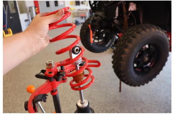
Step 8. Remove the OE main spring.
