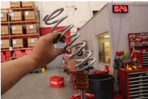
Step 17. Install Eibach tender spring.
