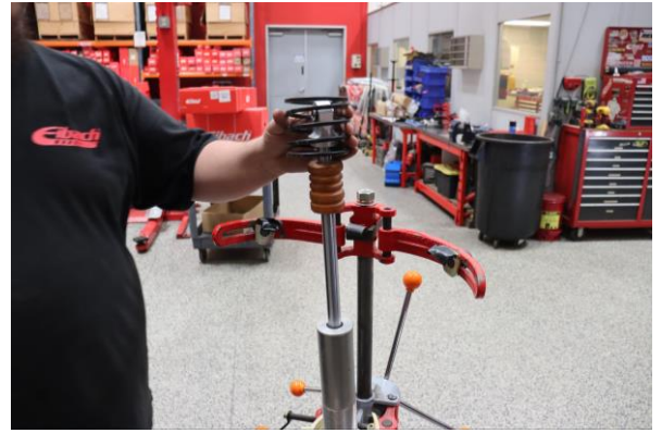
Step 14. Remove the second OE tender spring.
